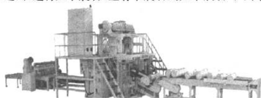
图2 数控有卡-无卡组合式一体机 Fig. 2 Chuck and spindleless combination veneer peeling machine
